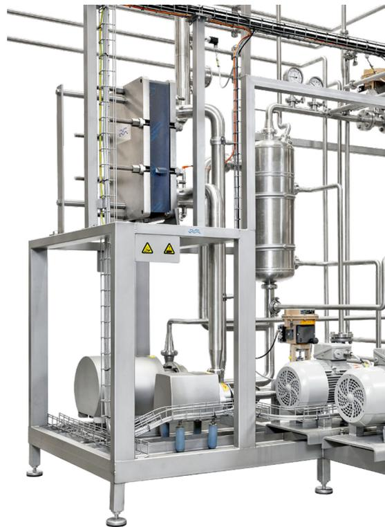
The De-alcoholization module's condensate cooling section.
