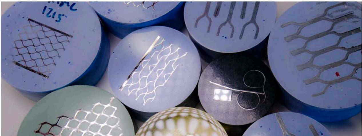
Molded samples with a mirrorlike surface for metallographic examination in a light optic microscope.
