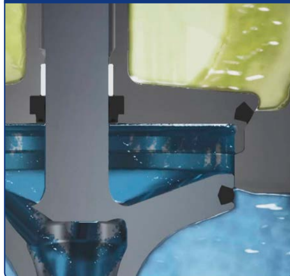
Figure 3. Seat push: The lower plug is pushed downwards thus cleaning the plug seal, seat and leakage chamber through CIP flow.
